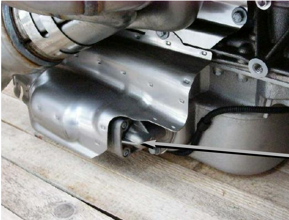
Electrically operated “duo-centric” oil pump (Left side shown)
